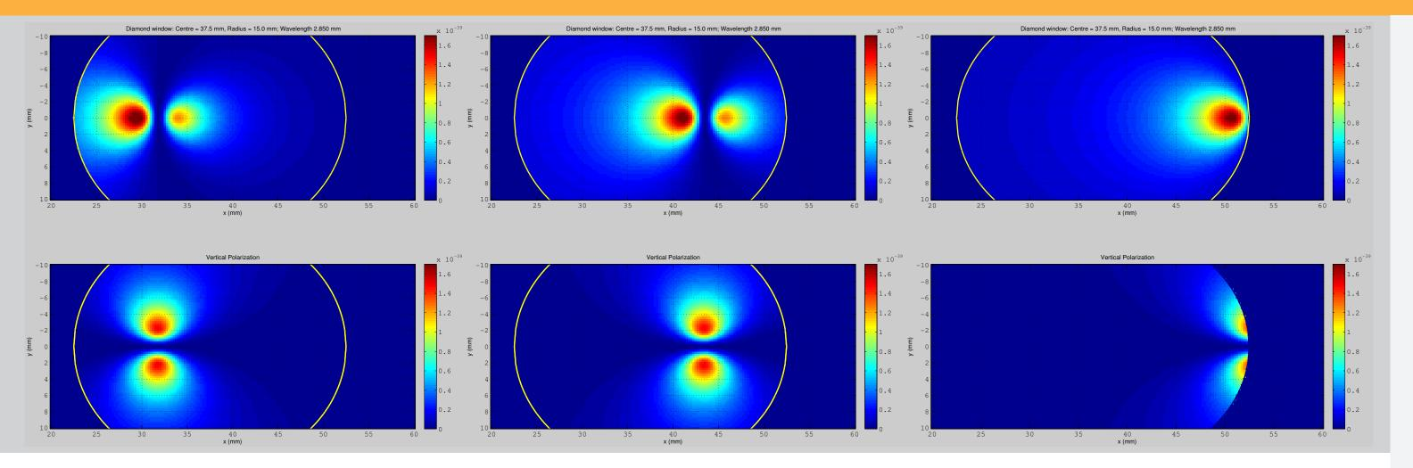
The synchrotron radiation distribution varies with bunch compressor angle. To assess these variations, the distribution on the vacuum window has been modeled. The system has been optimized for the nominal angle of 4.1°, but can be used between 3 and 5 degrees.
