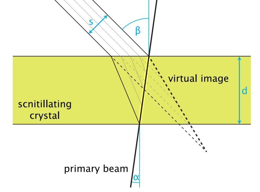
The primary beam produces a uniformly radiating slab of length d cos  $\alpha$ , which is observed at a distance much larger than d, under an angle  $\beta$  to the normal. We assume an index of refraction **n** in the crystal, surrounded by vacuum. Because of refraction on the surface of the crystal, the observer sees a virtual image of this slab, shown by a dashed line.
