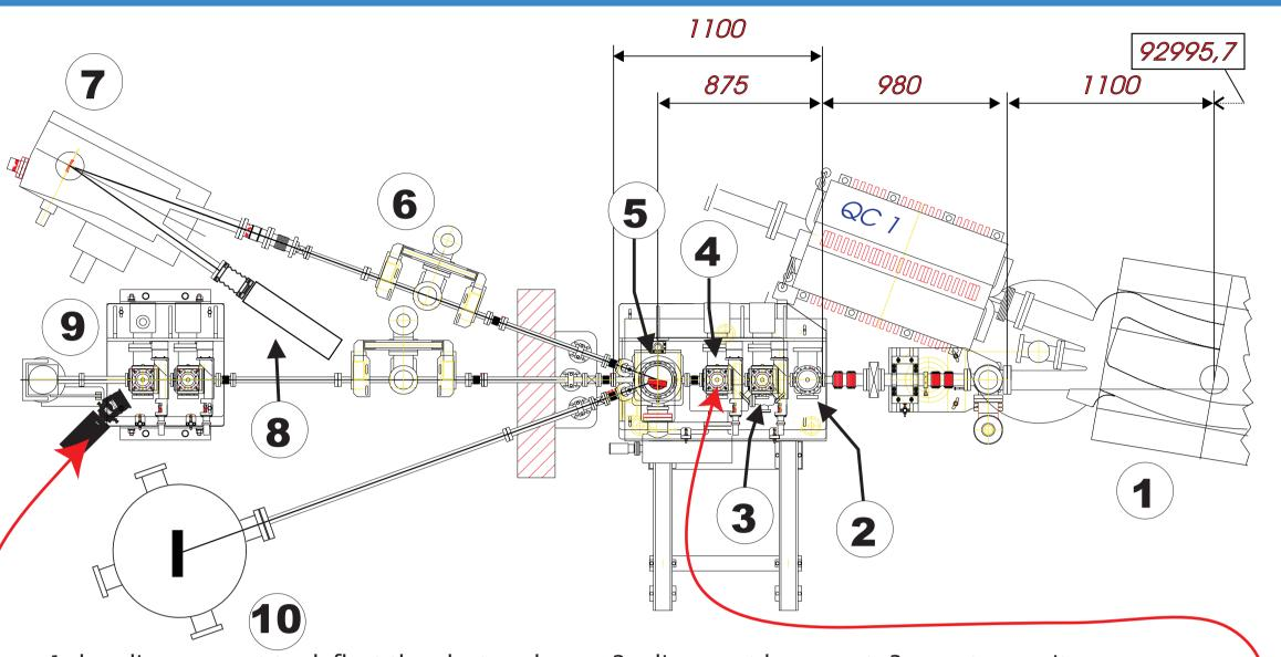
1: bending magnet to deflect the electron beam, 2: alignment laser port, 3: aperture unit, 4: detector and slits unit, 5: deflecting mirror, 6: TSP and ion getter pumps, 7: 1m normal incidence monochromator, 8: CCD-camera, 9: 2nd aperture and detector unit, 10: various experiments
