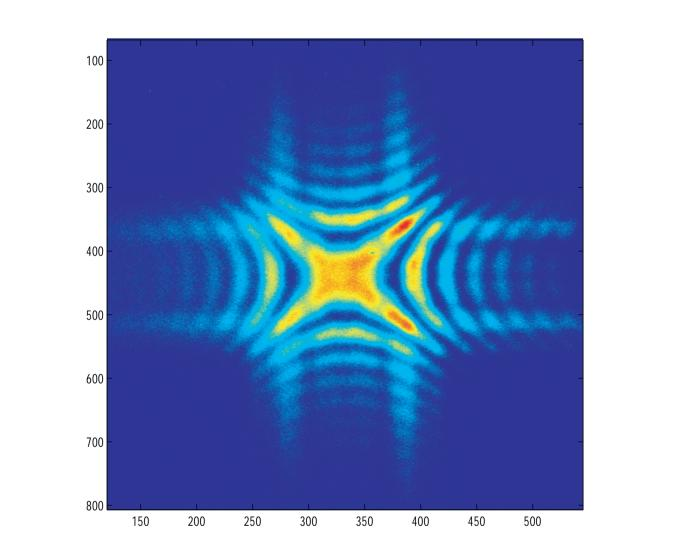
In principle, the crossed slits can be regarded as double slits with varying distance.
